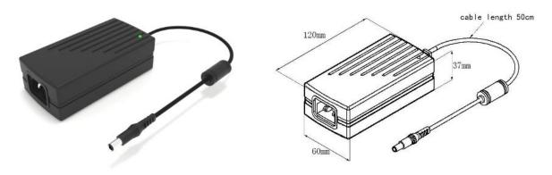
The Universal Diode Laser Module Power Supply with CE-marked provide a well-regulated 5VDC. This auto ranging power module can be connected to any 85-264 VAC 47/63 Hz supply. There is an IEC 60320 input socket and a 0.5m output cable terminated with an easy connect/disconnect jack socket. The Headset connector which could also be found in accessories is compatible with the power supply jack.
