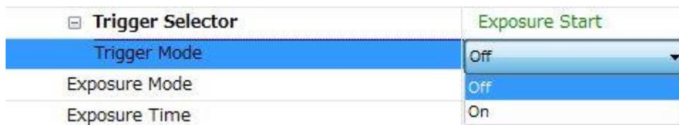
\* When this setting is enabled, it is necessary to supply a trigger packet from the frame grabber board to the camera.
