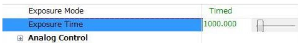
\* If increasing the ExposureTime setting, the value of AcquisitionLineRate may be changed automatically.
