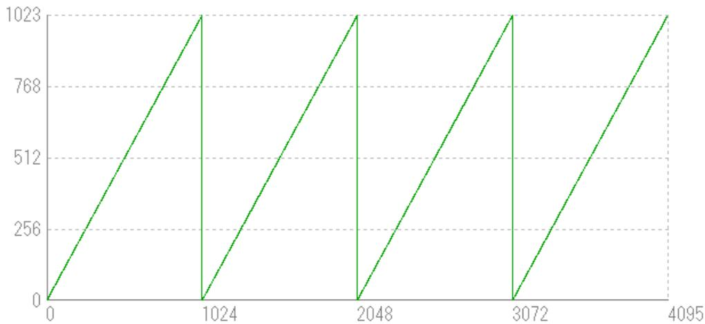
**Figure 4-10-4-3 Waveforms of the horizontal ramp pattern on Mono10**
