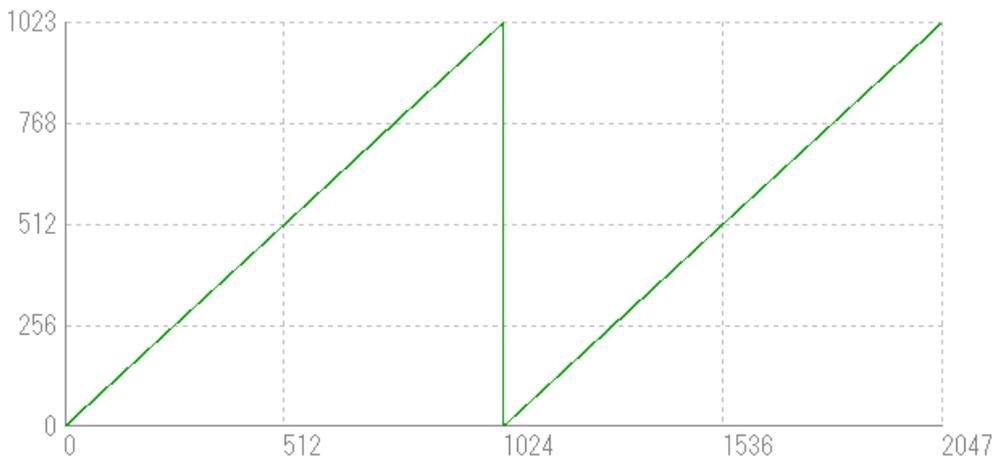
**Figure 4-10-8-3 Waveforms of the horizontal ramp pattern on Mono10**
