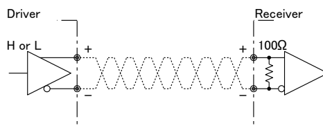
Figure 3-3-2 Circuit of LVDS
