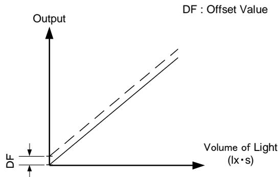
Figure 4-9-2 Offset Adjustment
