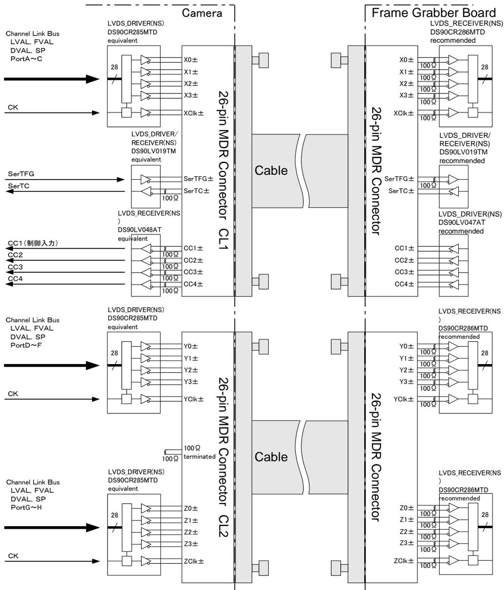
Figure 3-3-1 Camera / Frame Grabber Interface (Base, Medium)
