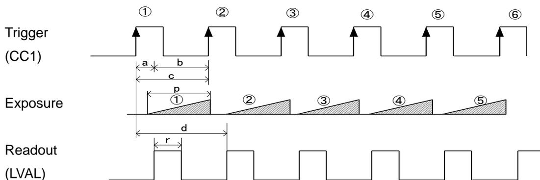
**Figure 4-8-2-1 External Trigger (Trigger Edge) Exposure Mode**
