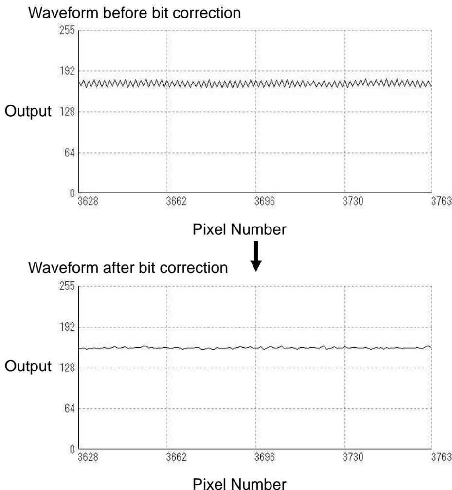
**Figure 4-11-1 Waveform before and after bit correction**
