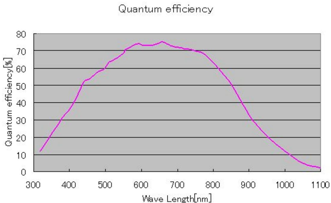
Figure 1-4-1 Quantum efficiency
