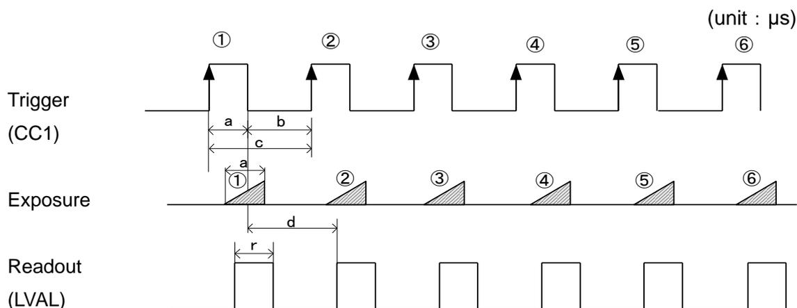
**Figure 4-8-3-1 External Trigger (Trigger Level) Exposure Mode**
