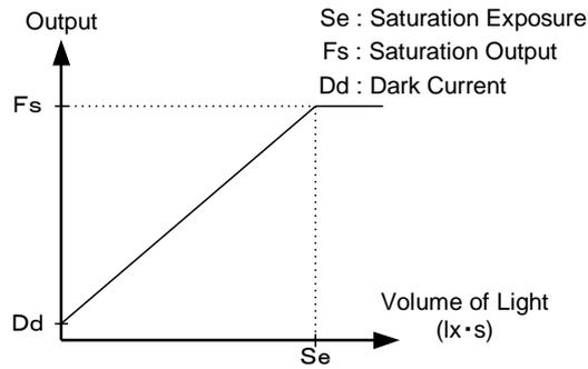
Figure 4-9-1 Saturation Exposure and Dark Current Output
