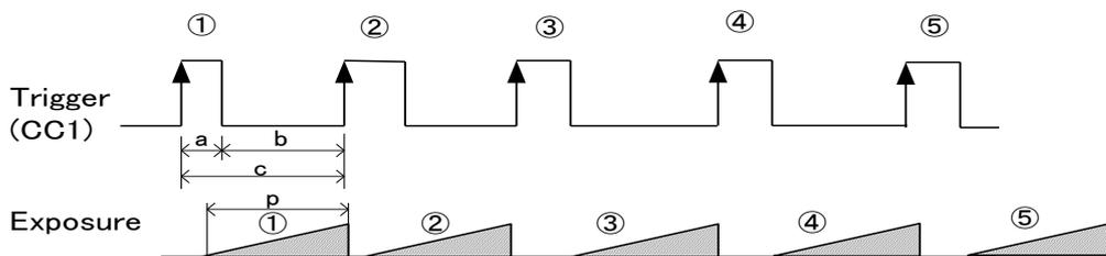
**Figure 4-8-2-1 External Trigger (Trigger Edge) Exposure Mode**
