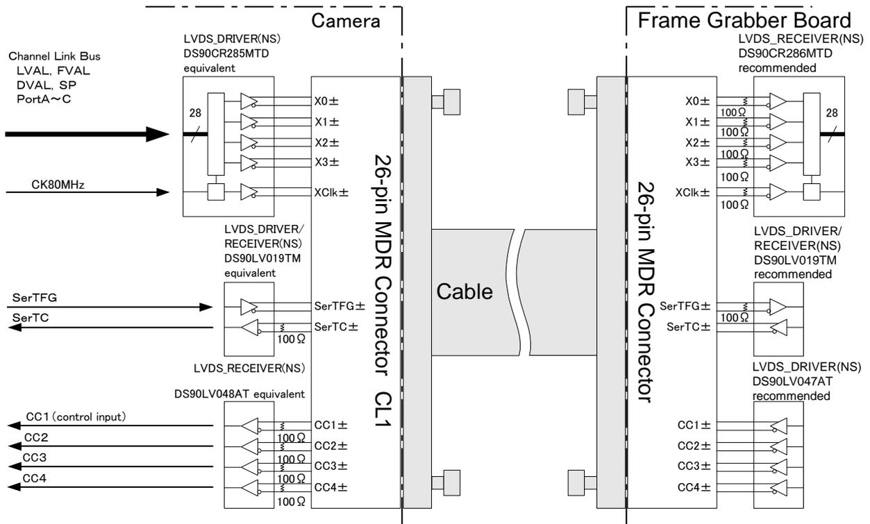
Figure 3-3-1 Camera / Frame Grabber Interface
