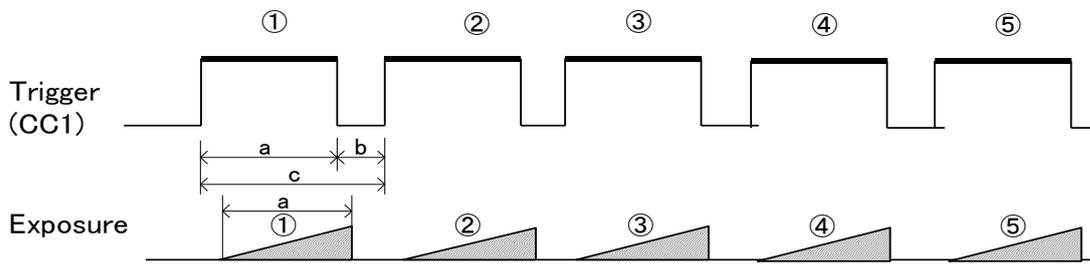
**Figure 4-8-3-1 External Trigger (Trigger Level) Exposure Mode**
