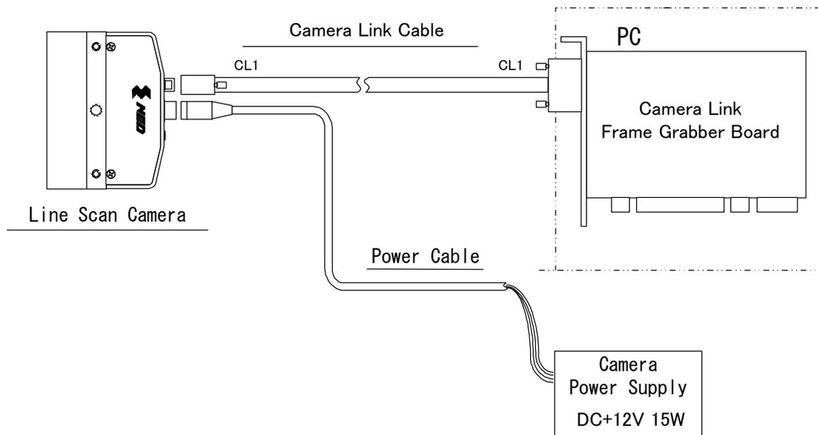
**Figure 3-1-1 Connections between Camera and Frame Grabber Board and Power Supply**
