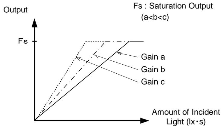
Figure 4-10-1 Gain Adjustment
