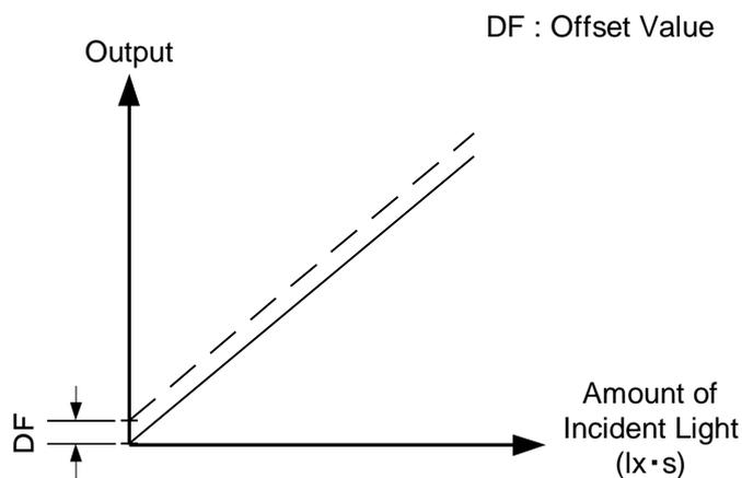
Figure 4-9-2 Offset Adjustment
