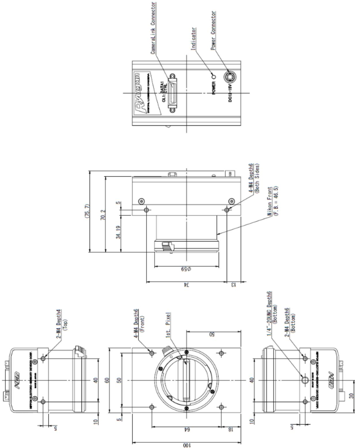
Figure 2-2-1 Dimensions of the Camera
