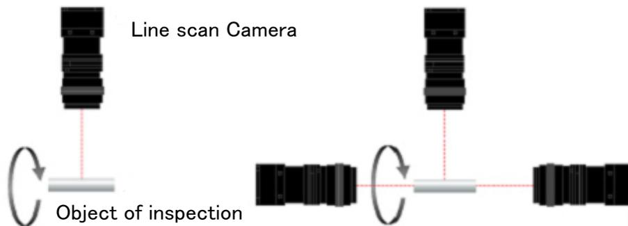
**Figure 1-2-1 Visual Inspection of Metallic Cylinder**
