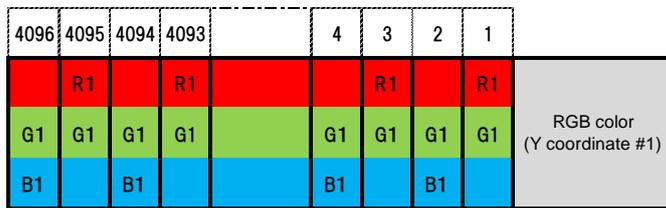
The values of R at even numbering pixels and B at odd numbering pixels are determined by interpolation.
