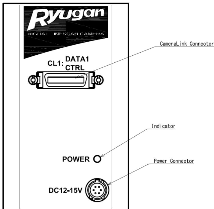
**Figure 3-2-1 Input/Output Connectors and Indicator**
