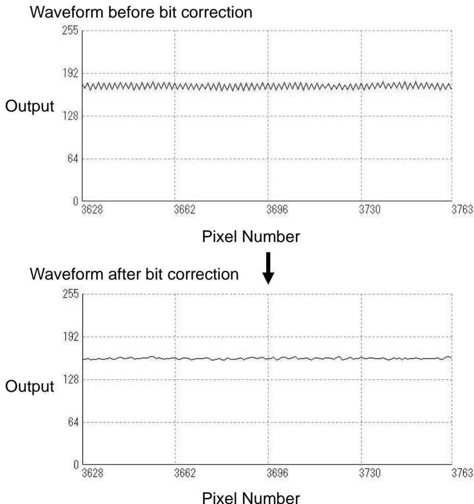
Figure 4-11-1 Waveform before and after bit correction
