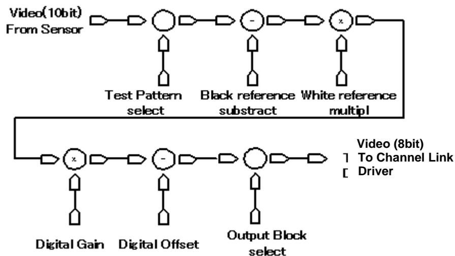
Figure 4-3-1 FPGA Processing Block Diagram
