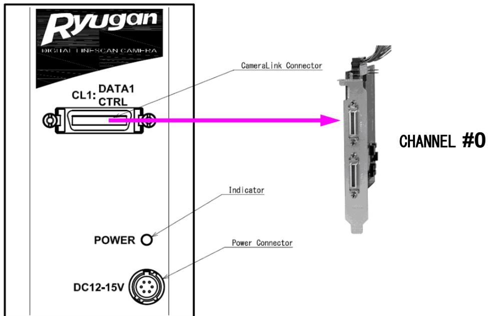
Figure 5-1-3 Channels of Camera Link Cables
