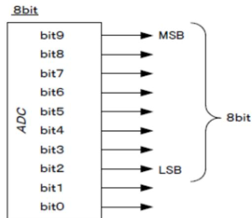
**Figure 4-7-1 Pin Assignments of Digital Data**
