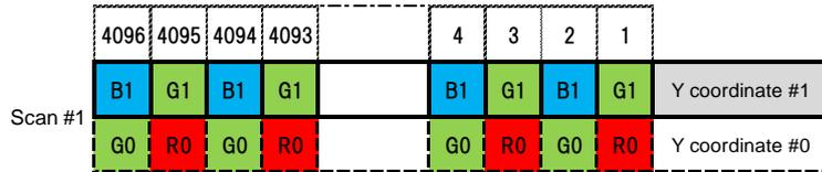
The object moves for one column of pixels and is scanned.
